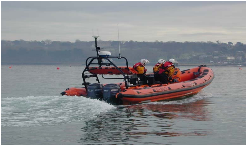
A new Atlantic 85 inshore lifeboat fitted with a pair of 4 stroke Yamaha 115HP Outboards, fully inversion-proofed, to be issued to coastal stations later this year.
